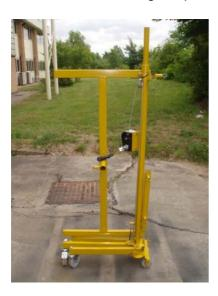
Once removed the plasterboard platform should be stowed at 90 degrees to the fixed castor leg in the transit channel. Ensure the locking pin secures the unit in position, as shown.
